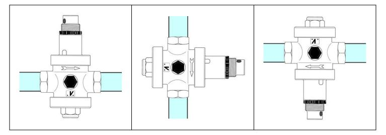
Pressure reducing valves can be damaged by dirty water; therefore we advise to install a self-cleaning filter upstream before the pressure reducer, in order to protect the valve and any other mechanism (thermostatic mixers, taps, etc.).
