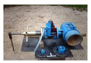
PERCAGE EN CHARGE SANS SOUDER ET SANS VIDANGER AVEC NOS OUTILS DE PRISE EN CHARGE
